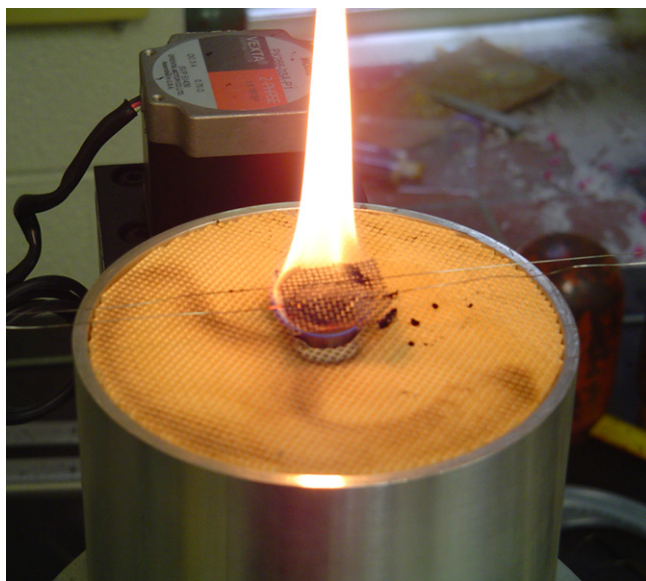
Fig. 1. Co-flow axisymmetric burner used for flame synthesis of CNSs.
